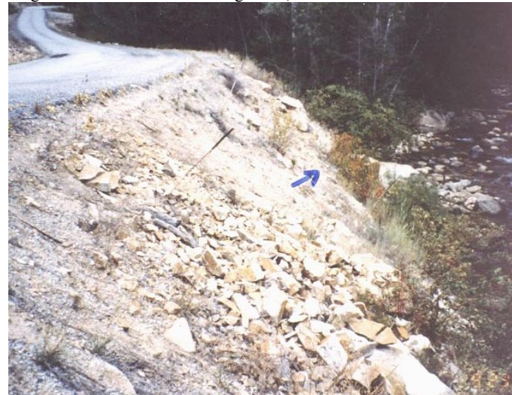
Photo 4. Eroding river banks with sparse cover of native plants killed or damaged (arrow) by spraying herbicide at stream. Sparse weeds on site (foreground) survived. Okanogan NF, WA.
